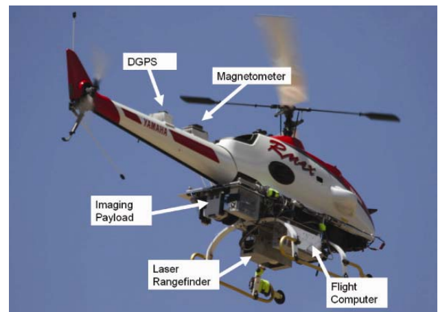
FIGURE 1. UNSW@ADFA R-Max in flight during laser-rangefinding experiments
