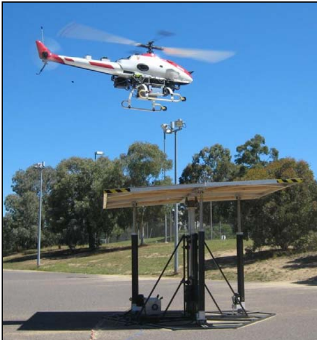
FIGURE 9. UNSW@ADFA R-Max hovering over moving deck simulator.
